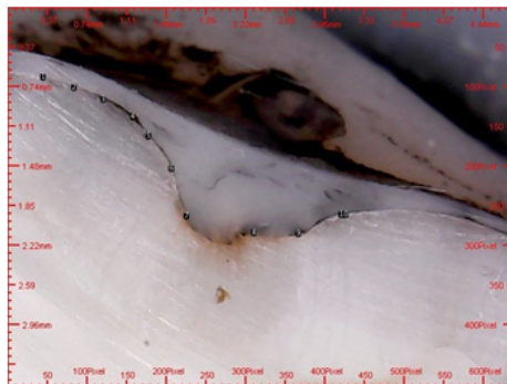
Fig.10 Optical microscopy measurements for dental probes with adhesive applied in a magnetic field for 5 min
